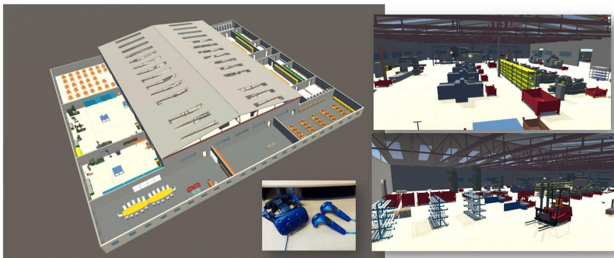
Fig. 2 Design of production system in virtual reality using HTC Vive Pro and Unity 3D
