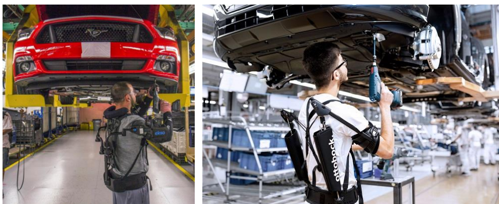
Fig. 1 Wearable upper body exoskeleton suitable for work overhead
