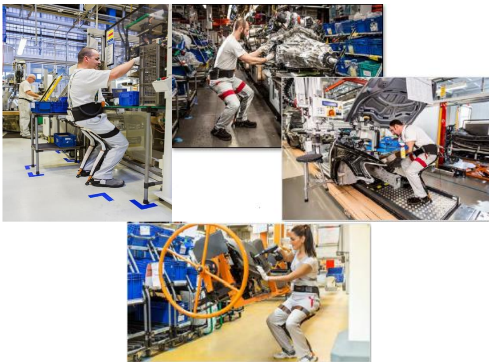
Fig. 3 Chairless chair exoskeleton in various working positions
