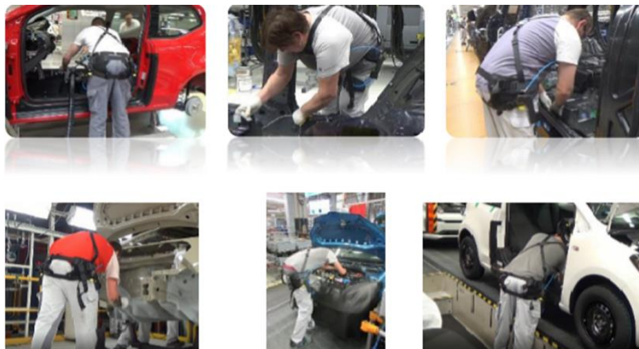
Fig. 2 Laevo exoskeleton in the testing phase in assembly operations
