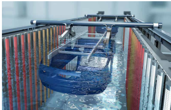
Fig. 7 Example of cataphoresis process
