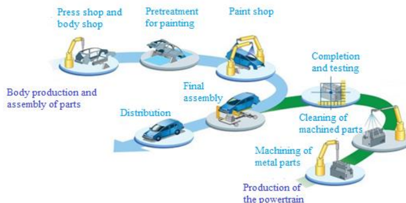
Fig. 3 The course of the main processes in the production of a car
