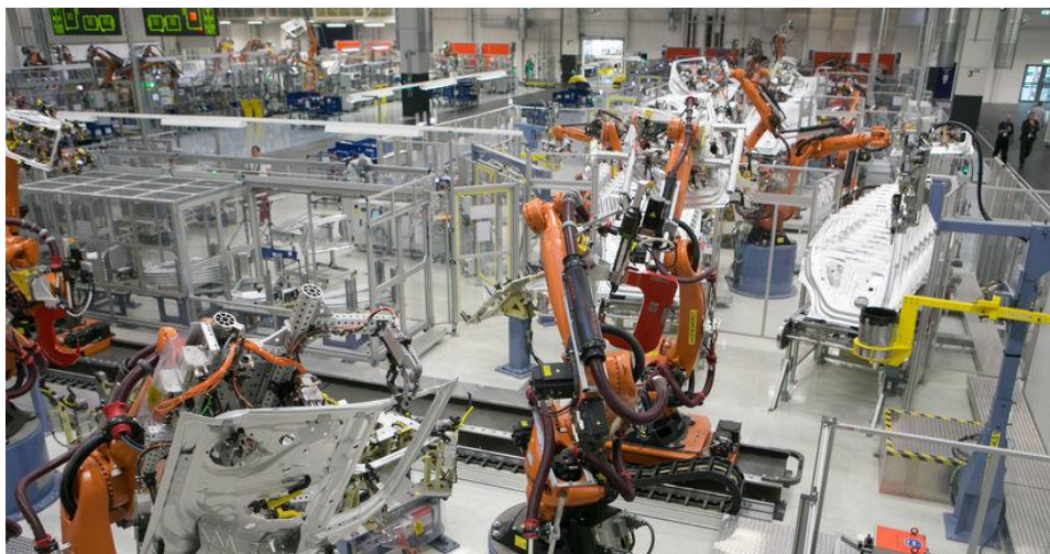
Fig. 5 Example of body shop with robots
